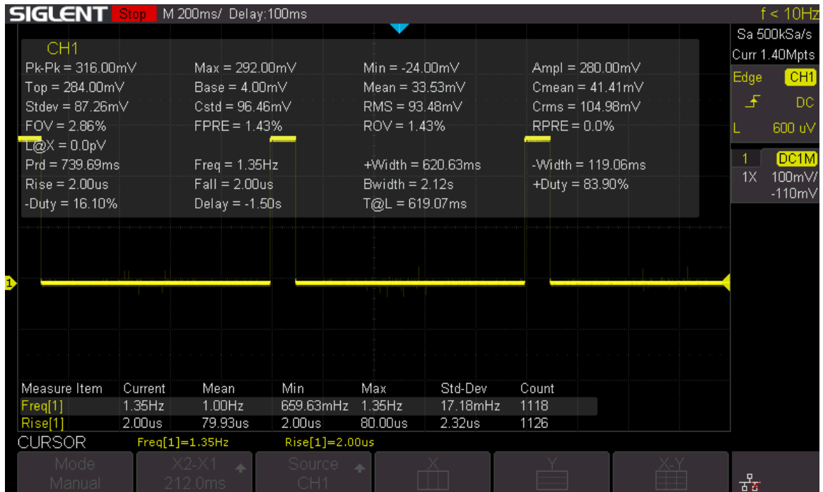
Figure 7: Signal information at ~1000 pulses from GPS receiver
